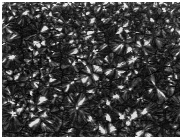
Fig. 4. HSOM image of PP spherulites after isothermal crystallisation at 130°C for 20 min, magnification × 100.
